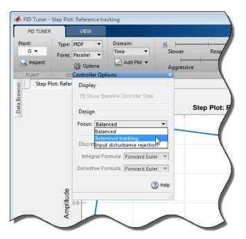
You can still use the **Response Time** and **Transient Behavior** sliders to further adjust the balance between reference tracking and input disturbance rejection.
